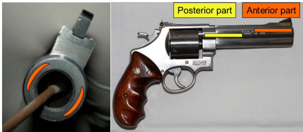
Fig. 1. Partial swabbing procedure: for the sampling procedure only half the circumference is swabbed, samples are taken separately from the front and rear end of the barrel.
